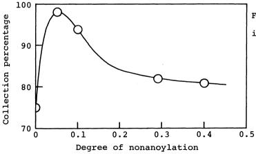
Fig. 1. Adsorption of copper (II) ion by nonanoylated chitosans.
